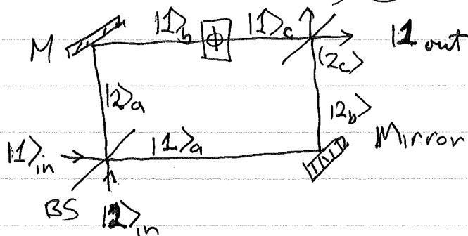
(a) We want to show that the MZ transformation on the two modes  $|1\rangle$  and  $|2\rangle$  ~~is~~ is equivalent to the SU(2) transformation on a 2D Hilbert space, as given in the assignment
